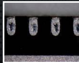
Typical wiping length 0.17~0.22mm
