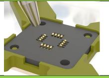
Use CDA to dry up excessive IPA to avoid staining on socket.
