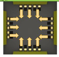
Sweep the pins gently with the nylon brush that was mildly soaked with IPA solution. Use the brush mildly soaked with IPA and brush along the pin tip in the direction as shown in yellow color.
