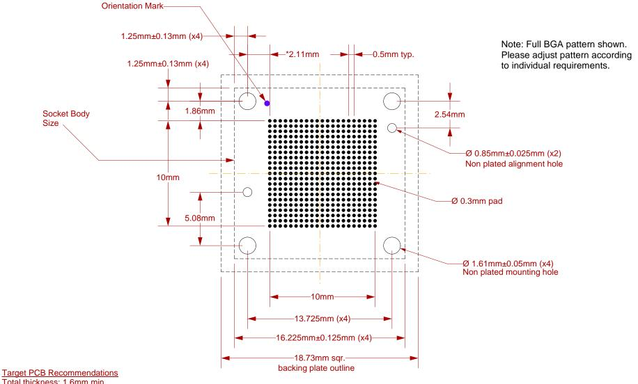
Total thickness: 1.6mm min. Plating: Gold or Solder finish PCB Pad height: Same or higher than solder mask
