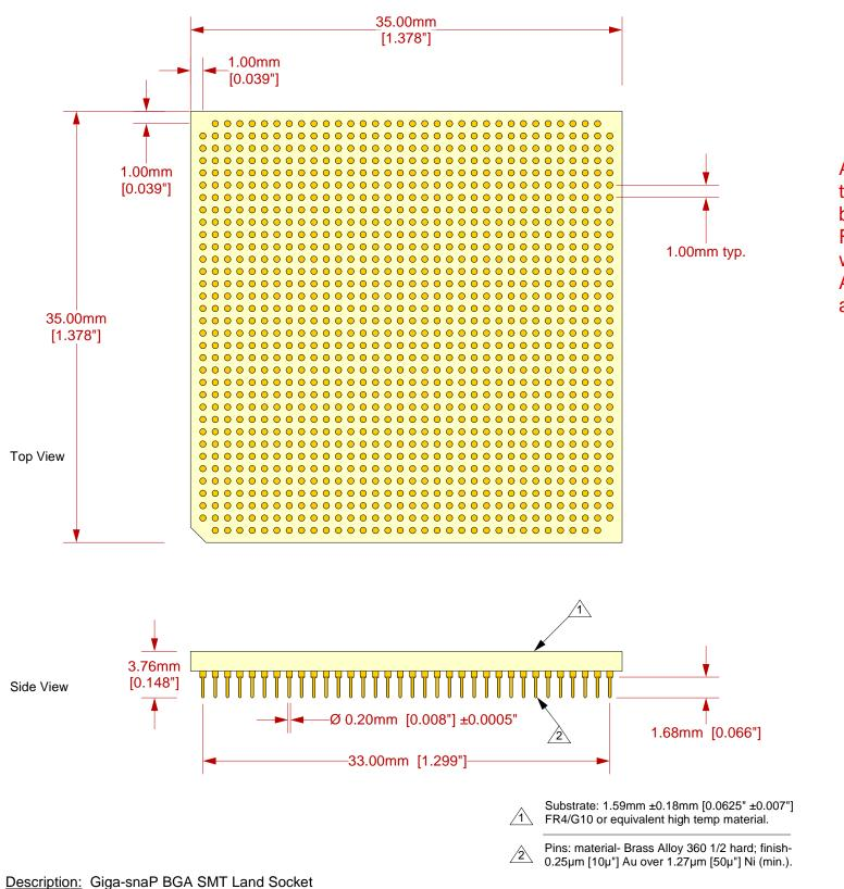
1152 position BGA surface mount land pattern to terminal pins (1.0mm [0.039"] centers, 34x34 array)
