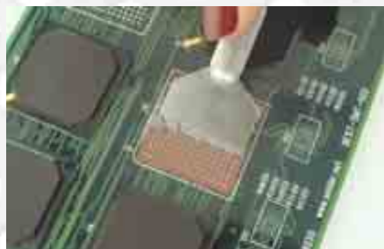
Step 3 - Squeegee paste or flux through the apertures onto the PCB
