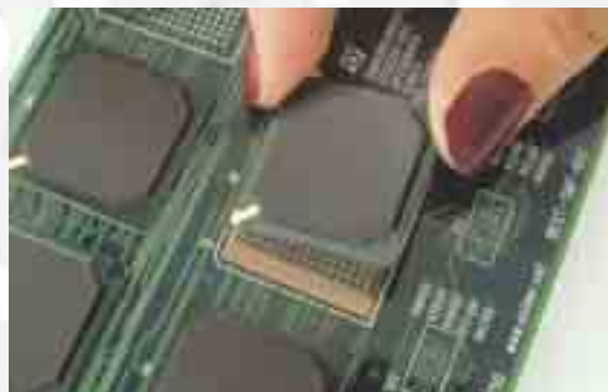
Step 4 - Align, place part and reflow
