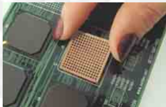
Step 2 - Align and affix the StencilQuik™ onto the PCB
