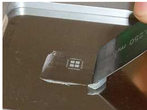
Figure 4: Squeegee solder paste
