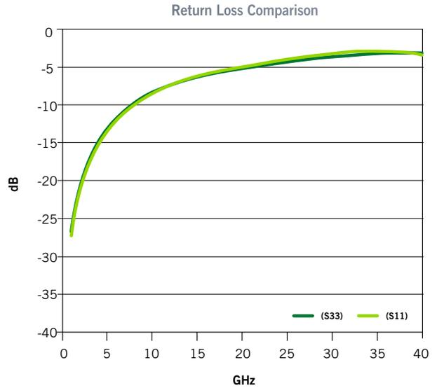
Figure 9. GSG P2A Return Loss comparison, 0.5 mm pitch
