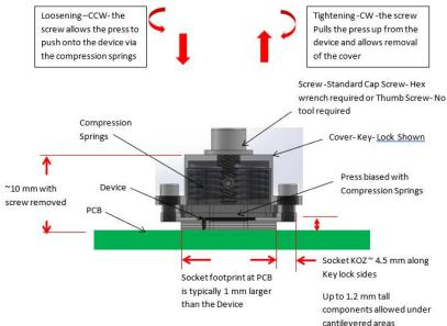
The example above shows a typical stack up of the lid. Optional designs for the lids are available that can be bolted to the socket body. Different designs have advantages and disadvantages based on the end application requirements; keep out zone (KOZ) considerations and nearby component heights. Ironwood can assist on your application to define the best socket and lid combination to meet your needs.
