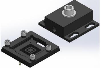
Grypper Y socket attaches the same as the Standard Grypper, G80 and G40 product through a reflow process. The Lid (shown left) locks to the shoulder screws in the socket frame. Once in place the screw on the top is turned counterclockwise which released the press onto the device. This screw can be left loose or removed
