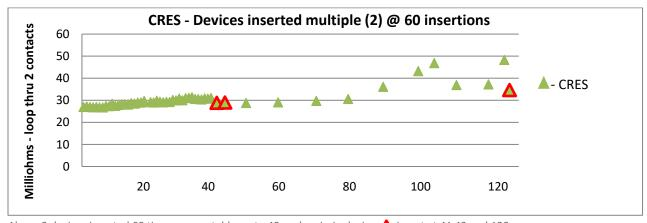
Above 2 devices inserted 60 times - very stable up to 40 each - virgin devices insert at 41 42 and 120
