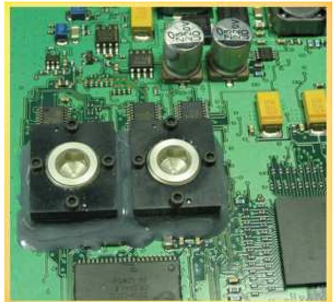
A clam-shell lid or swivel lid that allows quick removal and replacement of BGA packages can be integrated to the socket base structure while featuring the same space
