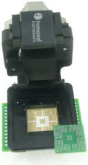
Figure 1: Clamshell BGA Socket using stamped spring pin contact.
