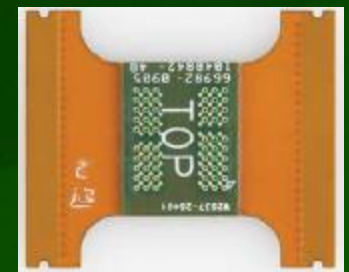
Two wing probe for DDR memory with optimized signal routing
