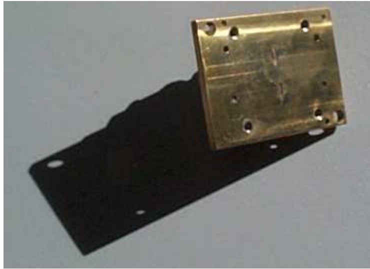
Figure 1 BGA 1.0mm socket base plate example
