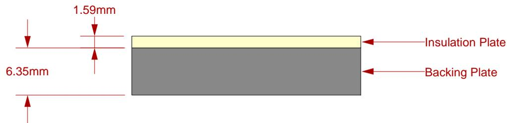
Description: Backing Plate with Insulation Plate
