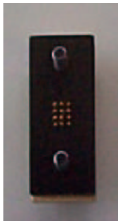
Fig. 2 Pin block with spring probe array
